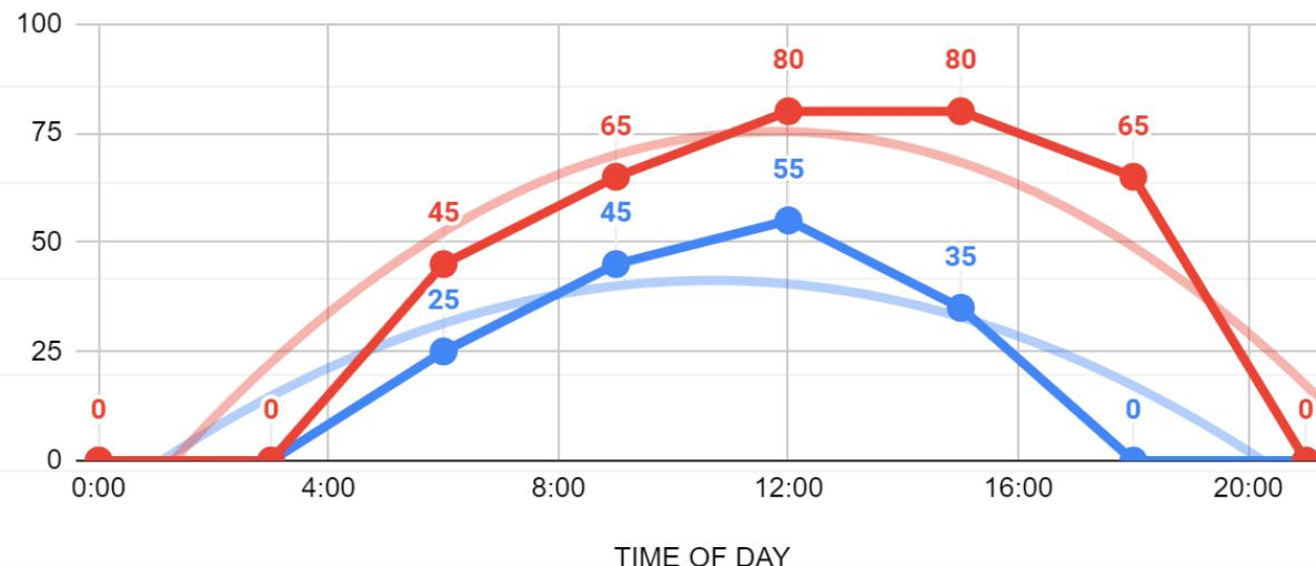
The difference in energy absorbtion when using a tracker and when without is significant.
